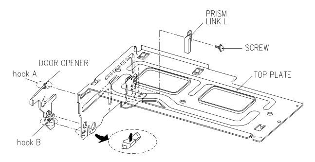
Fig. 3-4 DISASSEMBLY OF THE TOP PLATE
